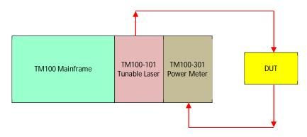
Using tunable laser and power meter to test optical component's characteristics, such as transmission or reflection spectrum, insertion loss, bandwidth, etc. Such as to test a DWDM filter.
