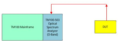
Fast scanning OSA (O-band or C-band) is an ideal instrument used in DFB laser diode (wafer level) screening test to measure the SMSR. With scanning speed as high as 50ms, it can dramatically improve the measurement cycle time and therefore the throughput.
